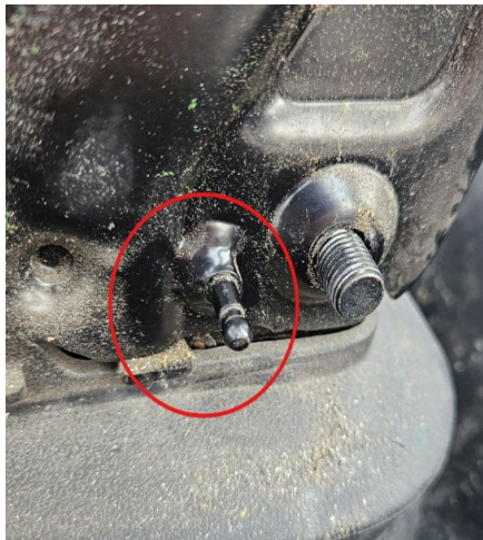
Figure 5: Locator Pin must be cut
