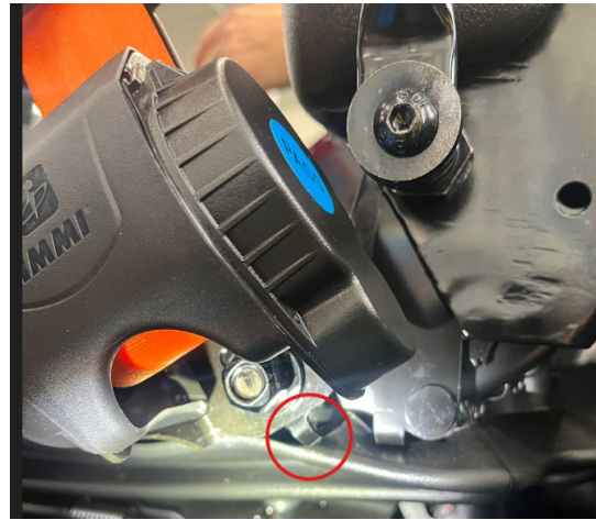
Figure 4: Alignment tab on Retractor
