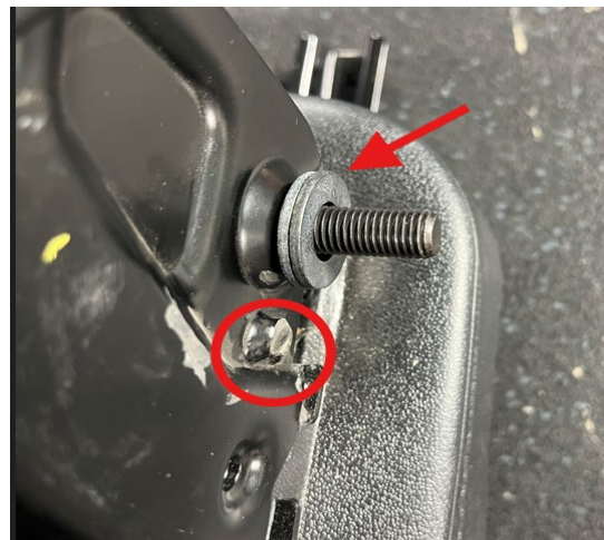
Figure 6: Cut Pin at first shoulder
